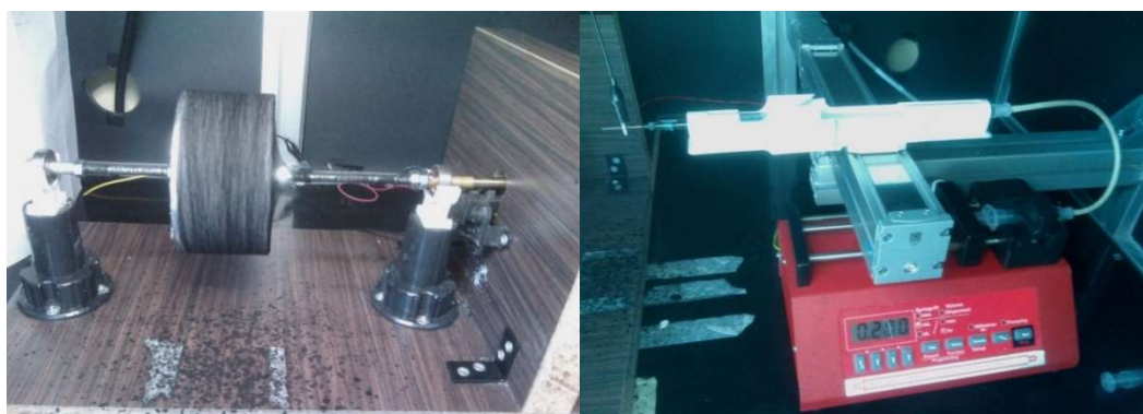
Fig. 1. Electrospinning setup: spinneret with syringe pump (right), collector drum (left)
